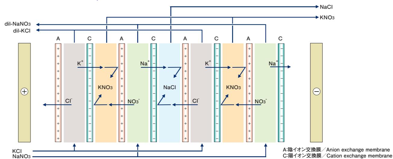
A:陰イオン交換膜 / Anion exchange membrane
